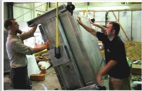
Rails for smooth, safe insertion of TPC into magnet
