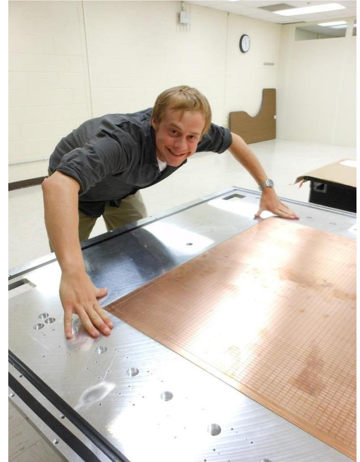
Testing the fit using an improperly manufactured board
