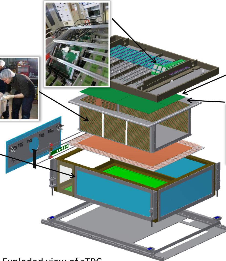
Wire planes amplify the electron signal, which is read out on the pad plane
