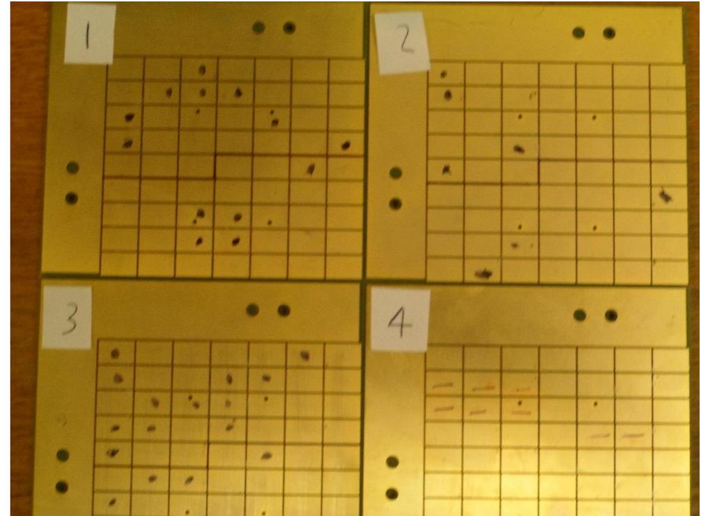
“Unit Cell” pad plane – Bad channels indicated with marker
