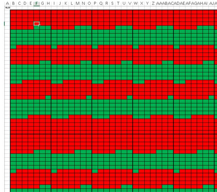
what if we lost one pad for every 2 star cards or 4 per every asad using this arrangement? We could use a 108\*112 pad arrangement and place one AsAd board in an array like this. (using the 4x12 arrangement for asad). This leaves room for STAR cards and a center crossing rib this uses 48 AsAd boards, the coding for every AsAd board would be the same, the coding for STAR boards would only require two different codes
