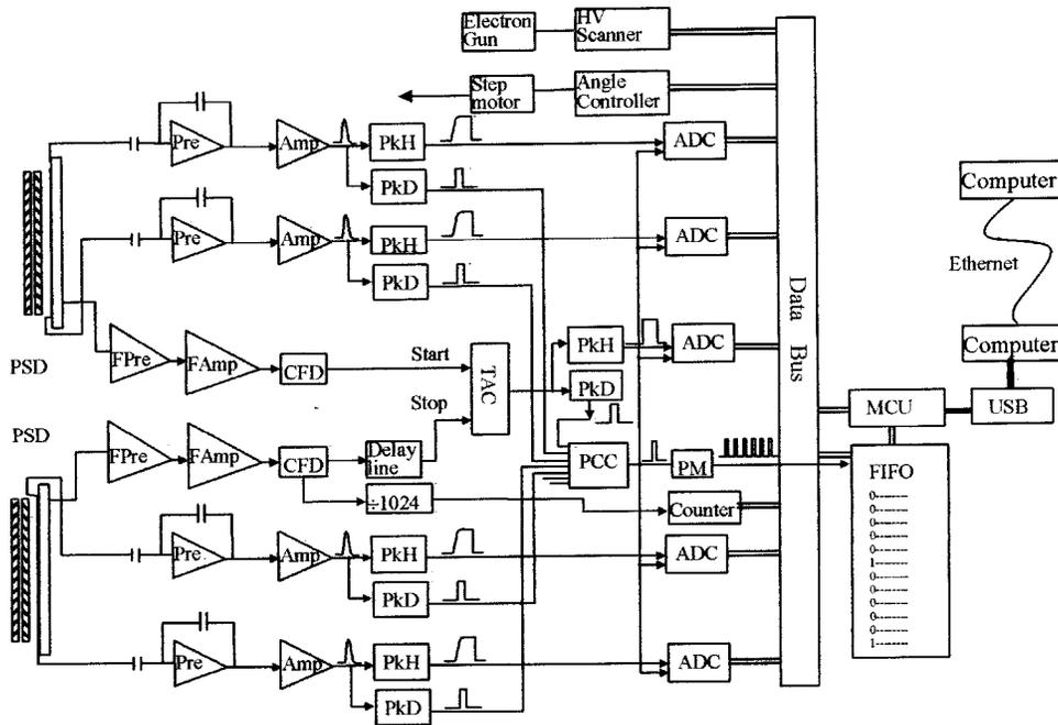
FIG. 1. Schematic diagram of multi-parameter acquisition system for the electron momentum spectrometer.
