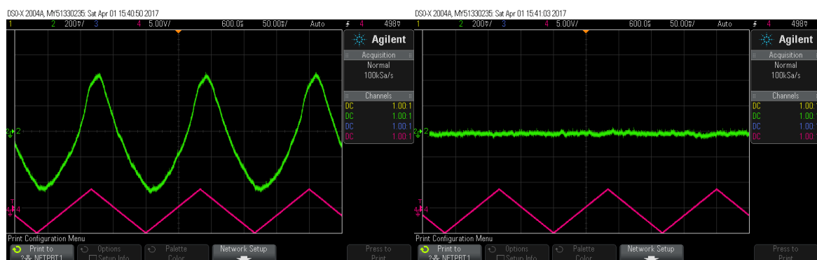
Fig. 4.15 The error signal before and after locking with the Yb hollow cathode lamp.
