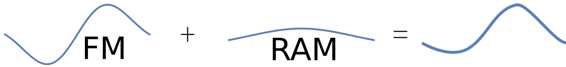
Fig. 4.13 The remained amplitude modulated (RAM) error signal. When the strong beam is modulated with the amplitude or direction, the resulted error signal will be asymmetric.
