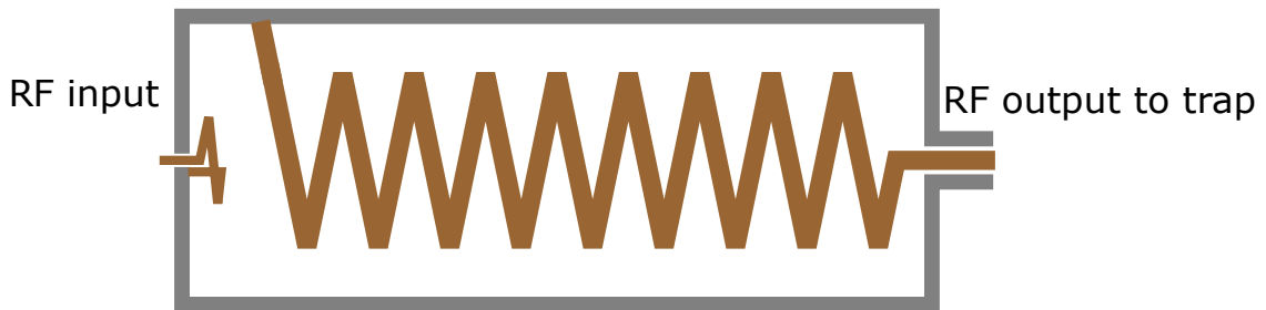
图 2.2 Schematic of helical resonator to show the inductive coupling between the RF input antenna and the trap electrodes.
