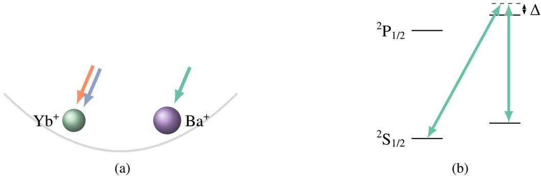
图 3.4 (a) Schematic representation of an open QRM realized by two ions. The red and blue arrow represent the detuned red and blue sideband laser respectively. The green arrow represent the lasers used in EIT cooling. The gray parabola schematically represents the trapping potential. (b) Energy levels of the Ba<sup>+</sup> ion that is related to the EIT cooling. Energy levels shown are not-to-scale.
