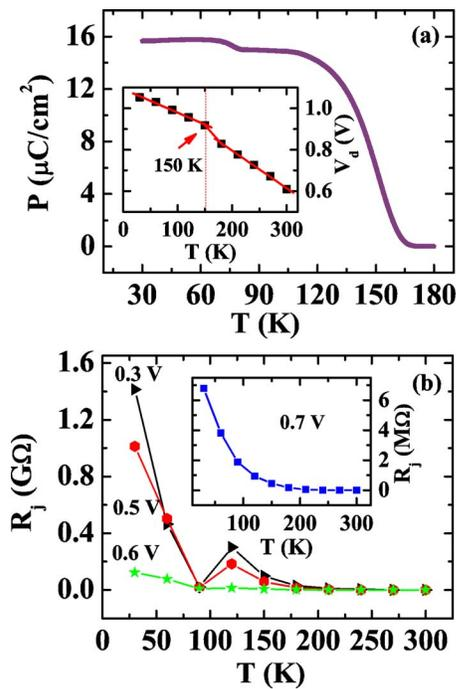
FIG. 2. (Color online) (a)  $P$ - $T$  curves of LBMO films. The inset is the temperature dependence of  $V_d$ . (b)  $R_j$ - $T$  curve for different forward bias voltages (0.3, 0.5, and 0.6 V) derived from the  $I$ - $V$  curves with different temperatures. The inset is the  $R_j$ - $T$  curve for 0.7 V.
