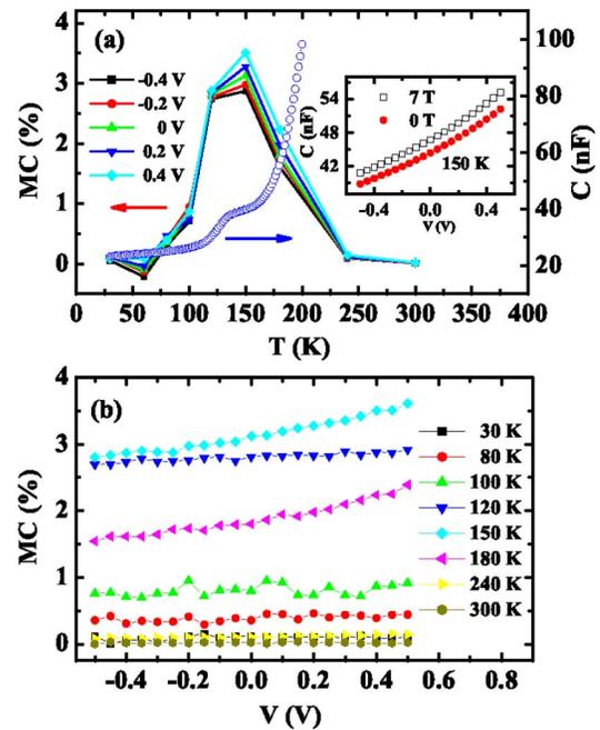
FIG. 3. (Color online) (a) Temperature dependence of the capacitance and MC. The inset is the  $C$ - $V$  curves measured at 150 K with and without a magnetic field. (b) MC- $V$  curves for samples at different temperatures.
