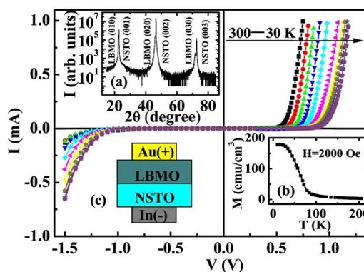
FIG. 1. (Color online)  $I$ - $V$  curves at different temperatures for LBMO/NSTO. The upper inset shows the XRD pattern for LBMO/NSTO. The right bottom inset is the temperature dependence of magnetization of 75 nm LBMO films. The left bottom inset is the layout of the device for measurement.
