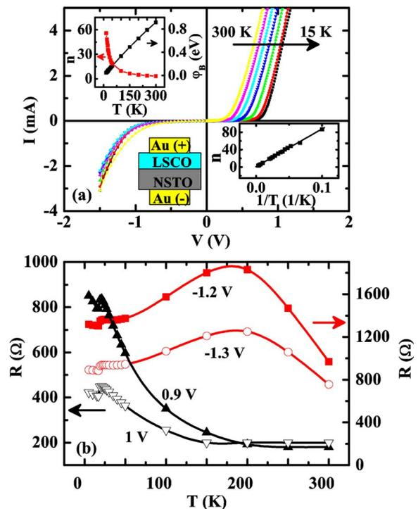
FIG. 1. (Color online) (a)  $I$ - $V$  curves of LSCO/NSTO at different temperatures (300, 250, 200, 150, 100, 50, and 15 K). The top inset shows  $n$ - $T$  and  $\phi_B$ - $T$  obtained from the  $I$ - $V$  curves. The left bottom inset is the layout of the device for measurement. The right bottom inset is the  $n$ - $1/T$  curve. (b)  $R$ - $T$  curves with different bias voltages.
